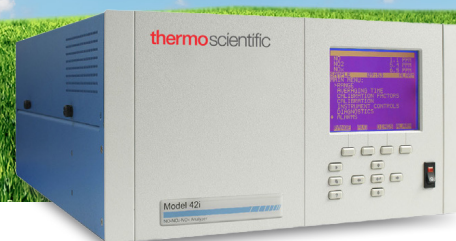
Model 42i NO-NO 2 -NO x Analyzer
